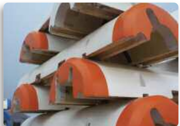
Client's drilling riser buoyancy modules after repair
