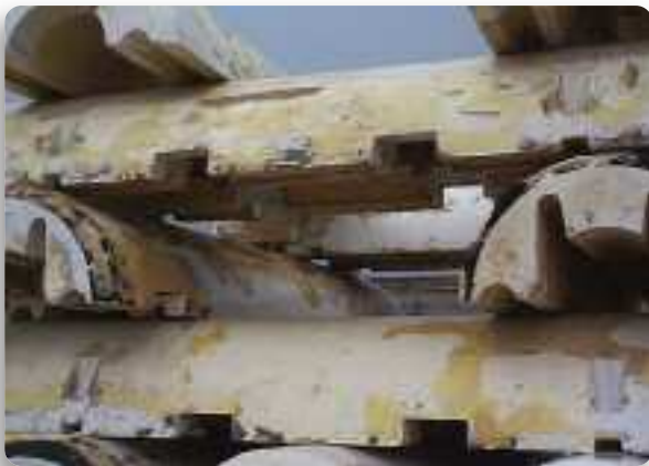
Client's drilling riser buoyancy modules before repair
